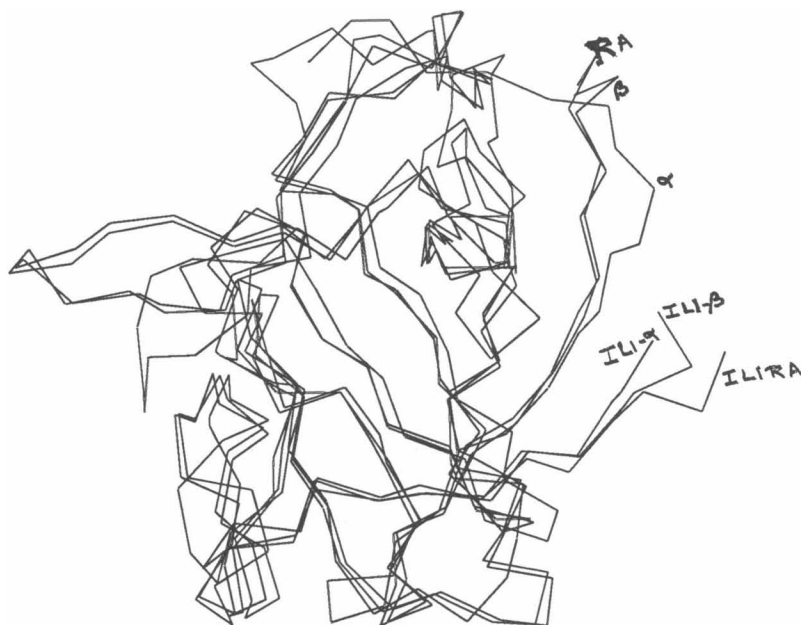
FIGURE 2 Superposition of the \alpha -carbon backbones of IL1 \alpha , IL1 \beta and IL1RA.
